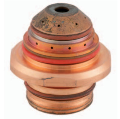
THERMACUT NOZZLE AFTER 6 HOUR CUTTING
