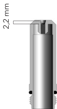
Maximum wear of the all-silver electrode 2,2 mm deep
