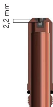
Maximum wear of Thermancut SILVER PRO electrode 2,2 mm deep
